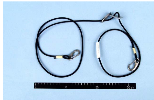
Figure 9.7-15 Russian flat bungees (left), U.S. large adjustable round bungee (right).
